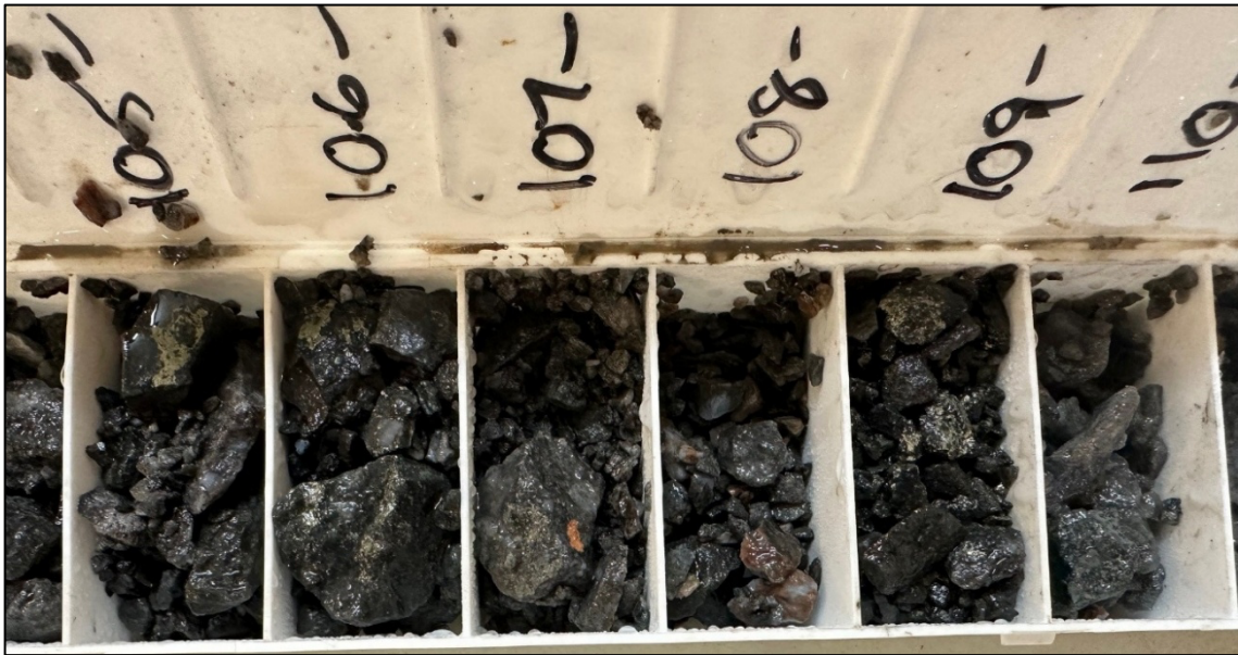
Figure 4. Logged sulphides and quartz veining CWRC25-43. Maximum 1m assays; gold 0.02 g/t Au, arsenic 31 ppm and copper 431 ppm.
