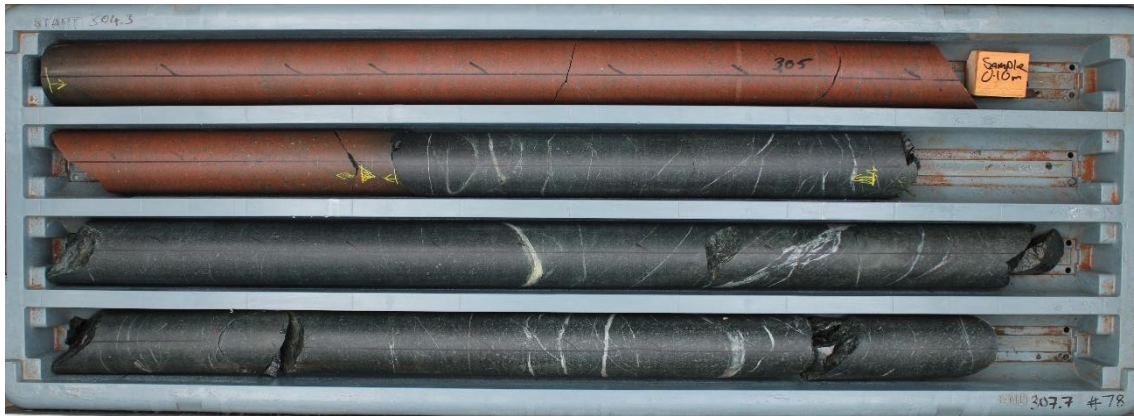
Figure 7. HDD26-01 logged apatite (reddish orange) indicating proximal felsic intrusion a potential driver of mineralised fluids.
