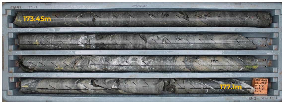
Figure 6. Shear zone with quartz veining / breccia with pyrite stringers and silicification of basalt. Anomalous pathfinders 3.65m @ 61.66 ppm As, 0.44 ppm Bi, 9.7 ppm Mo, 3.04 ppm Sb and 0.2 ppm Te from 173.45m. Similar geology; alteration, structurally and pathfinder element anomalism occur throughout the depth of the hole.
