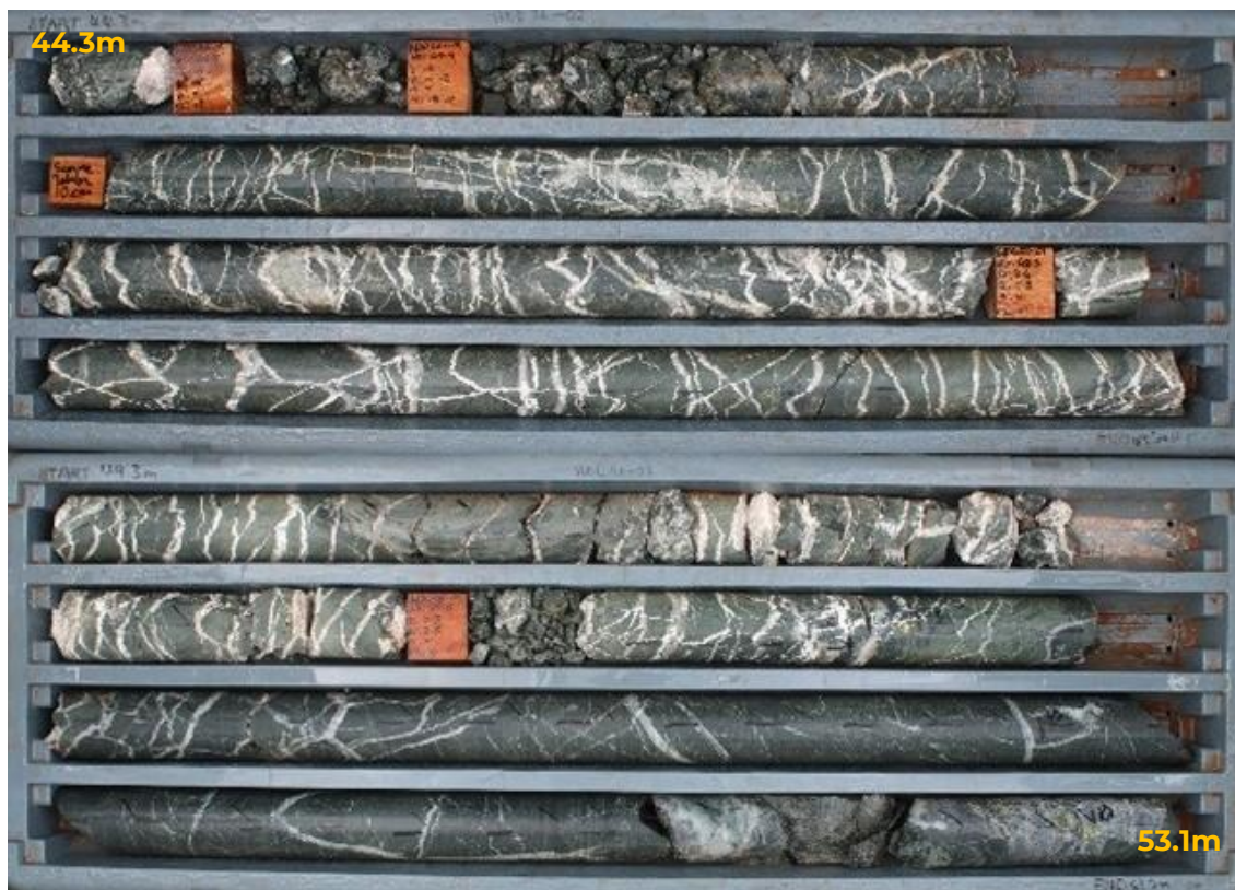
Figure 5. HDD26-01 – showing intense quartz-carbonate veining occurring within at least two phases of alteration. Depth 44.3m to 53.1m
