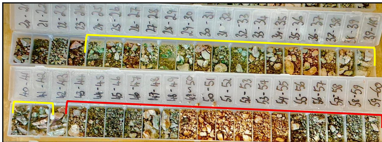
Photo 1: RC drill chips from hole MBDD003 at MB4 IP/MAG Target. Yellow brackets approximate main copper zone to date & red brackets quartz dominated alteration zone with traces of copper.
