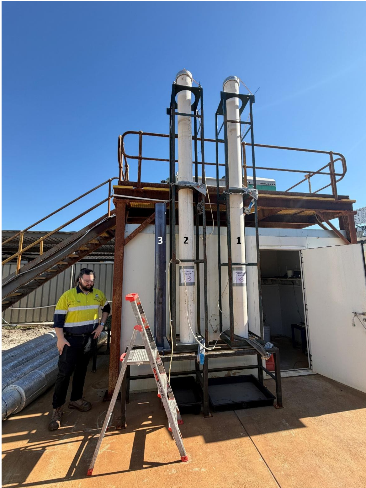
Figure 4 - Columns One, Two and Three Under Leach
