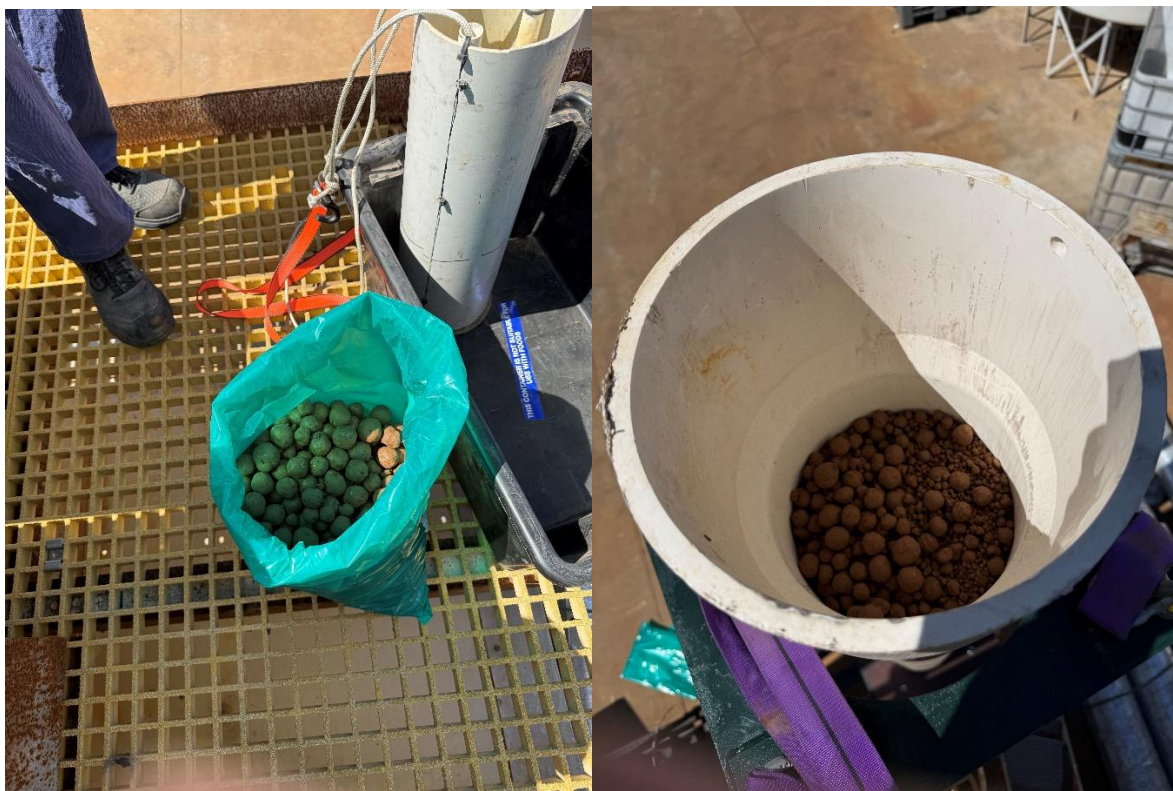
Figure 3 - Column two leach agglomerates on the left and inside the column on the right
