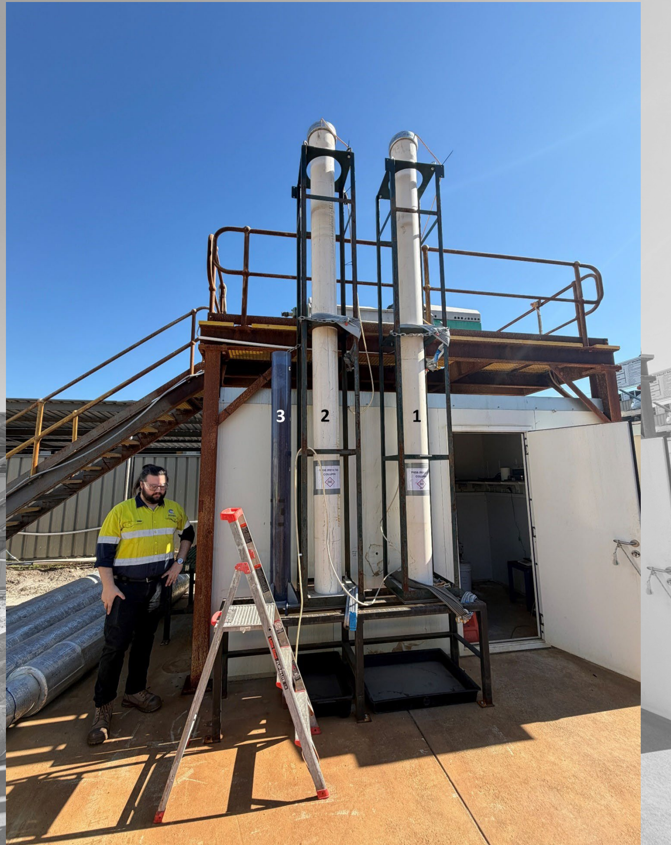
Column Leach testwork at IMO Laboratories proving up Heap Leach recoveries and performance
