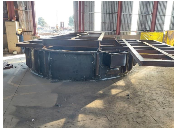
Figure 9: CIL Tank fabrication
