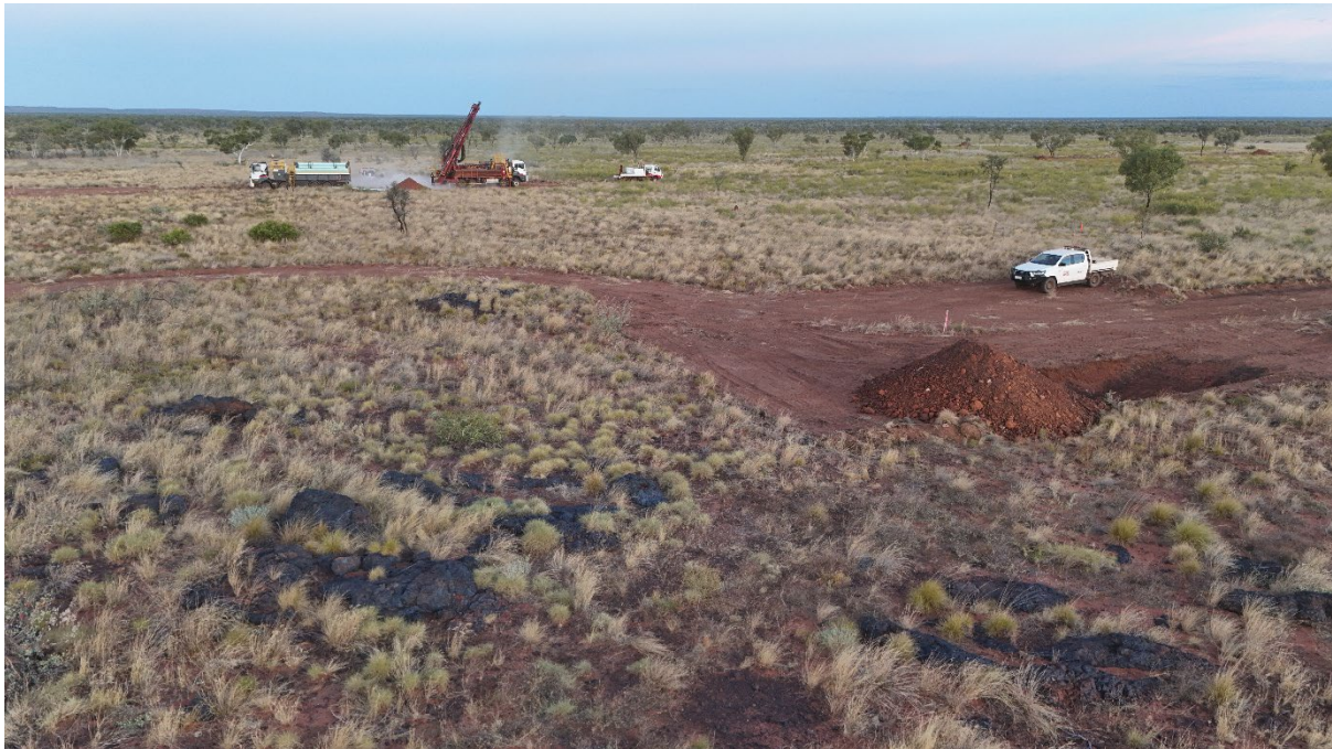
Figure 2. Precision Exploration Drilling (PXD) Reverse Circulation drill rig on the first hole with manganese outcrop in the foreground.
