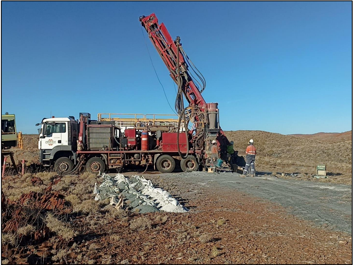
Figure 1 RC rig on-site at Tambourah King.
