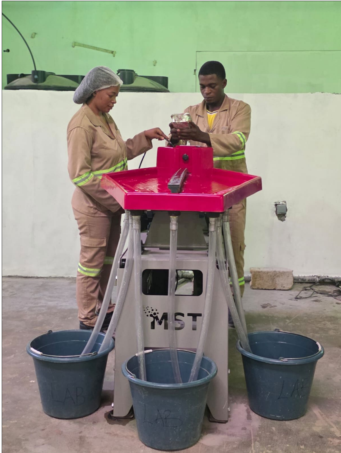
Figure 1: Tusker lab technicians processing exploration samples over the shaking table.
