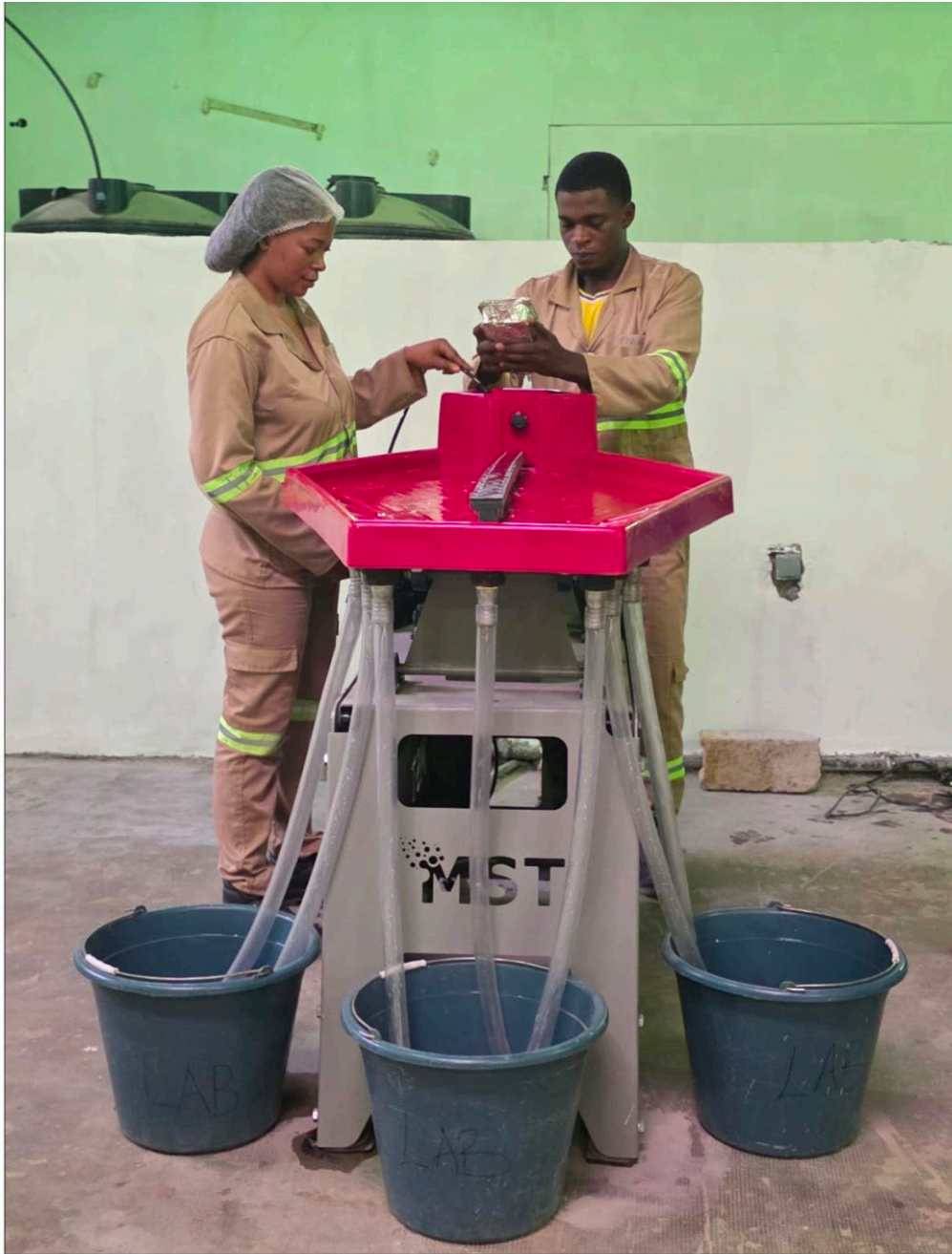
Figure 3: Tusker lab technicians processing exploration samples over the shaking table at the Yaoundé HMS laboratory. (ASX Announcement, 10 March 2026.)
