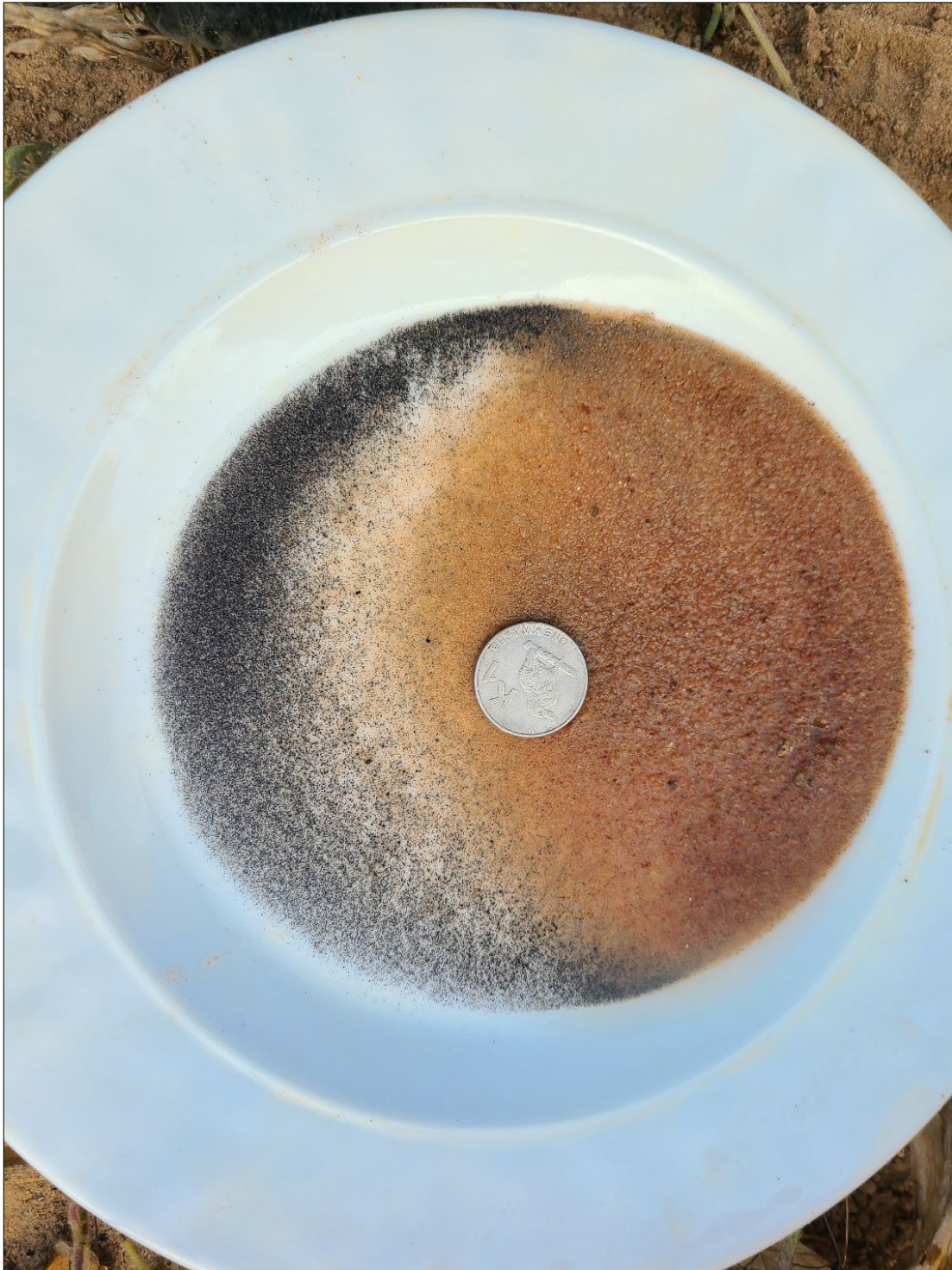
Figure 4: Panned fine grained heavy mineral concentrate recovered from Pit 6 (0–1 m; UTM Zone 36S: 543644E, 8679301N) demonstrating abundant heavy mineral content with accessory quartz, minor kyanite, garnet and mica.
