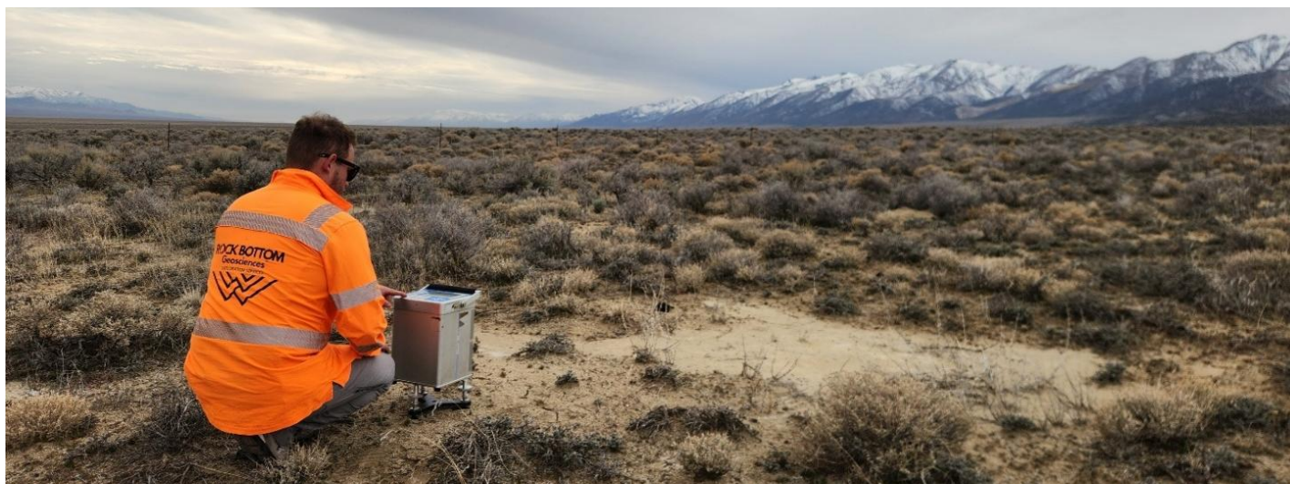
Figure 15; Photo showing field data collection using a Scintrex CG 5 gravimeter at the Linka Project, Nevada, USA.
