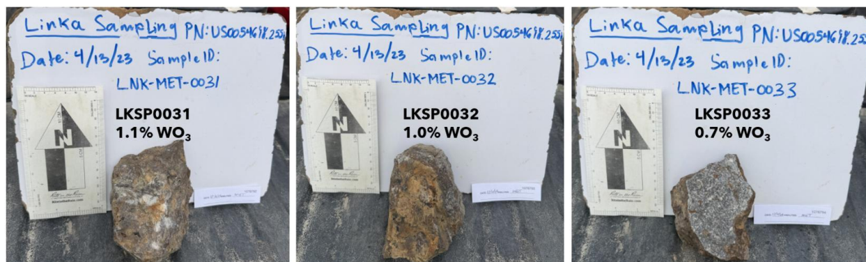
Figure 3: Photo showing high grade samples collected from the Linka stockpile. Grade annotated on the image. Refer to Figure 2 for location and data tables for sample coordinates.
