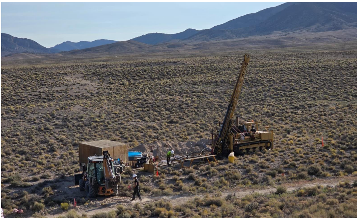
Figure 1. Diamond drill rig set up over drill-hole RMDD009 (Plan ID RMP006)
