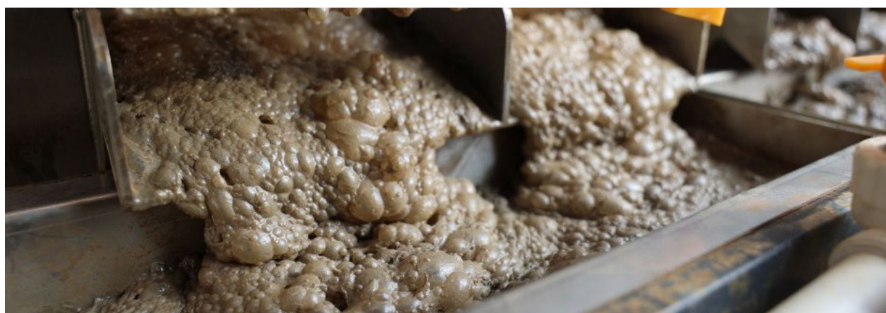
Figure 32: Froth Formation During Pilot-Scale Flotation Testwork
