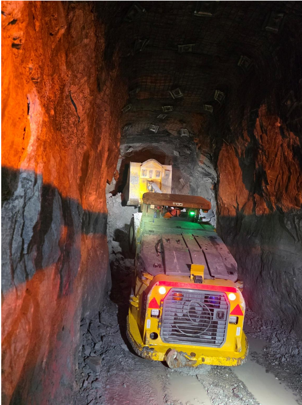
Figure 5: The stopes will be bogged out using the remote controlled Aramine loaders
