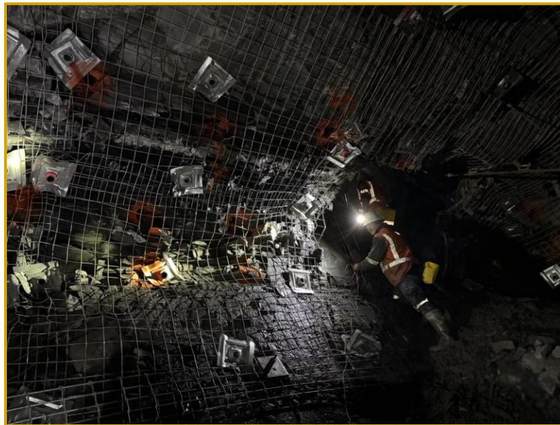
Figure 2 : The 8m longhole slot rise at Decline 3, Mica 1 lens, following the trial stope's first firing
