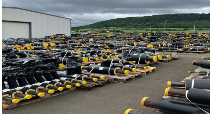
ICPP pipe connections at pipe fabrication yard in Germany.
