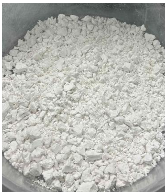
Figure 4: Hydrated niobium oxide precipitate (before calcination)
