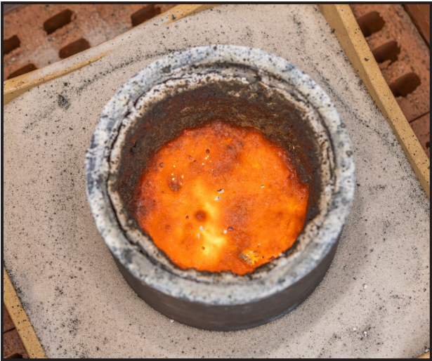
CONVERSION VESSEL COOLING FOLLOWING FERRONIUMIUM TESTWORK
