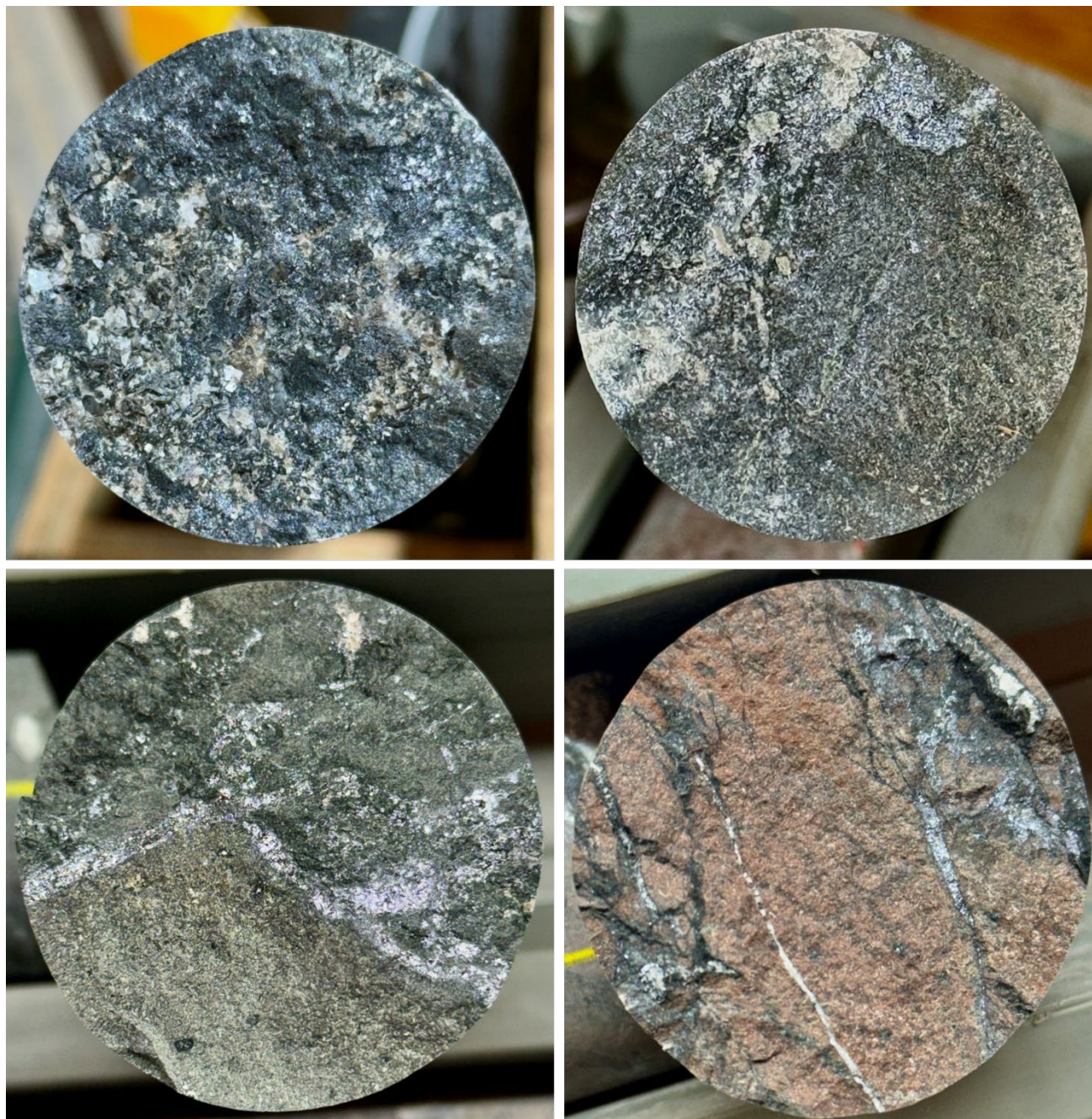
Figure 4 - Photographs of NQ2 diameter diamond drill core. Clockwise from top left depths are 208m, 211m, 229.3m, 241.1m. Images show variably altered (chlorite and hematite) chalcocite bearing basalts. Chalcocite forming breccia cement and veinlets with calcite and chlorite.
