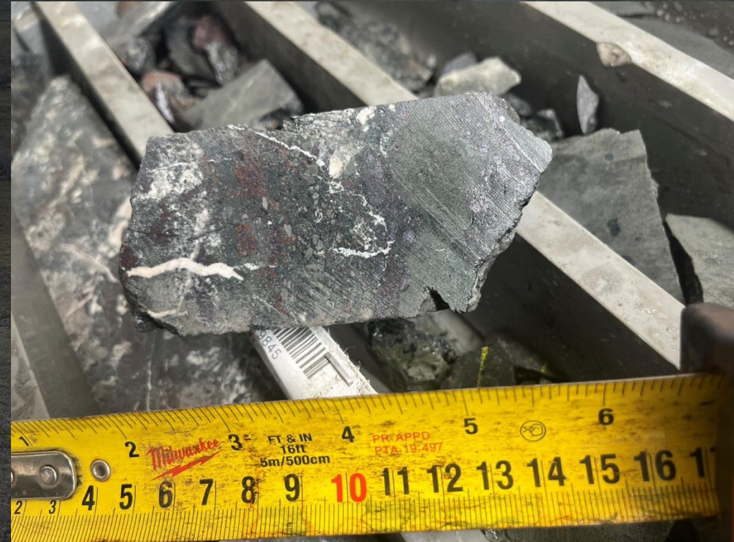
Figure - Photograph of halved NQ2 diameter core showing mixed chalcocite and bornite mineralisation in the chlorite breccia zone at 45.5m in DAN26026
