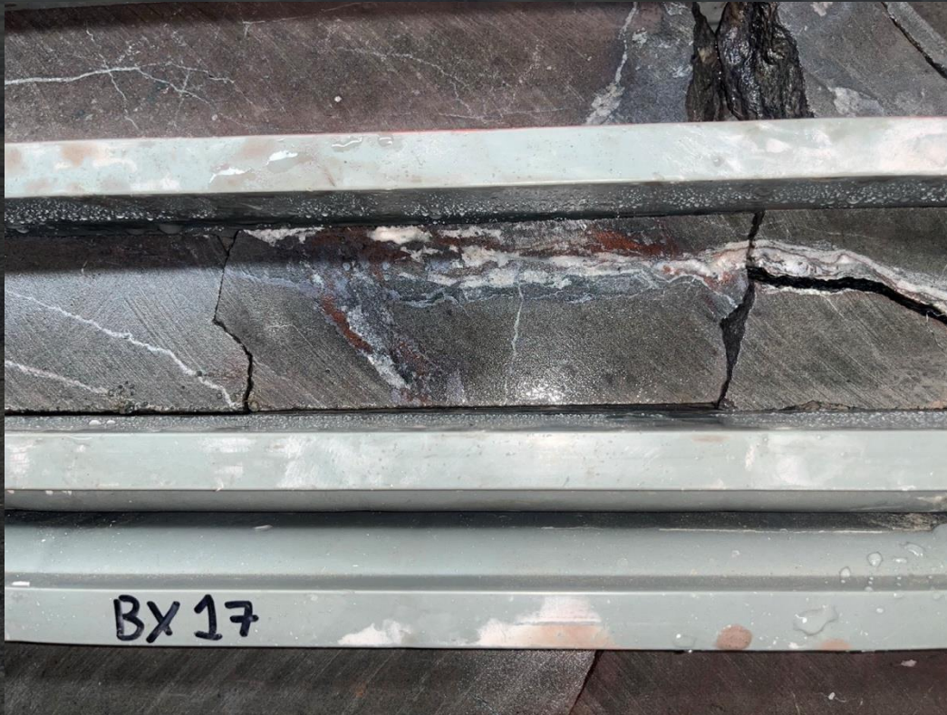
Figure - Photograph of cut NQ2 diameter core containing vein-hosted chalcocite from 66.4m downhole in DAN26026
