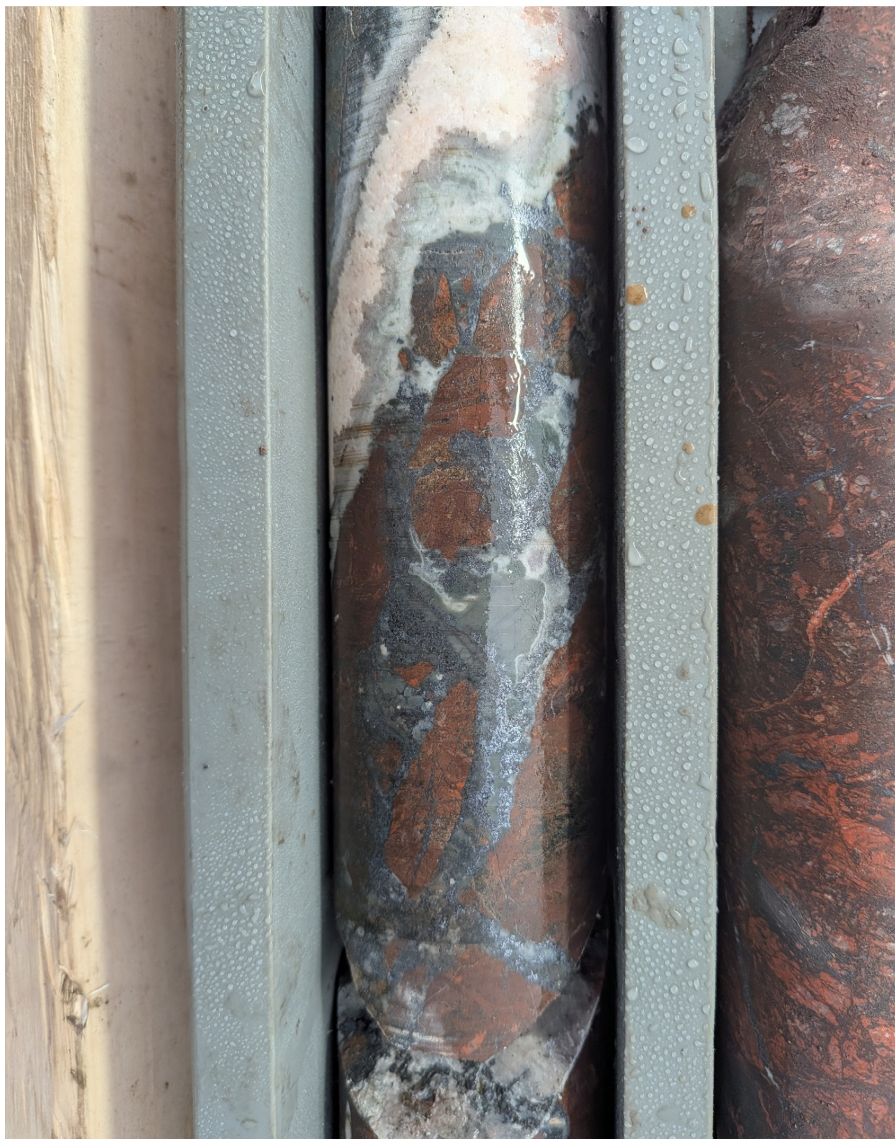
Figure 7 - Photograph of chalcocite veining from 168.5m in DDH DAN26031. Core is NQ2 diameter.
