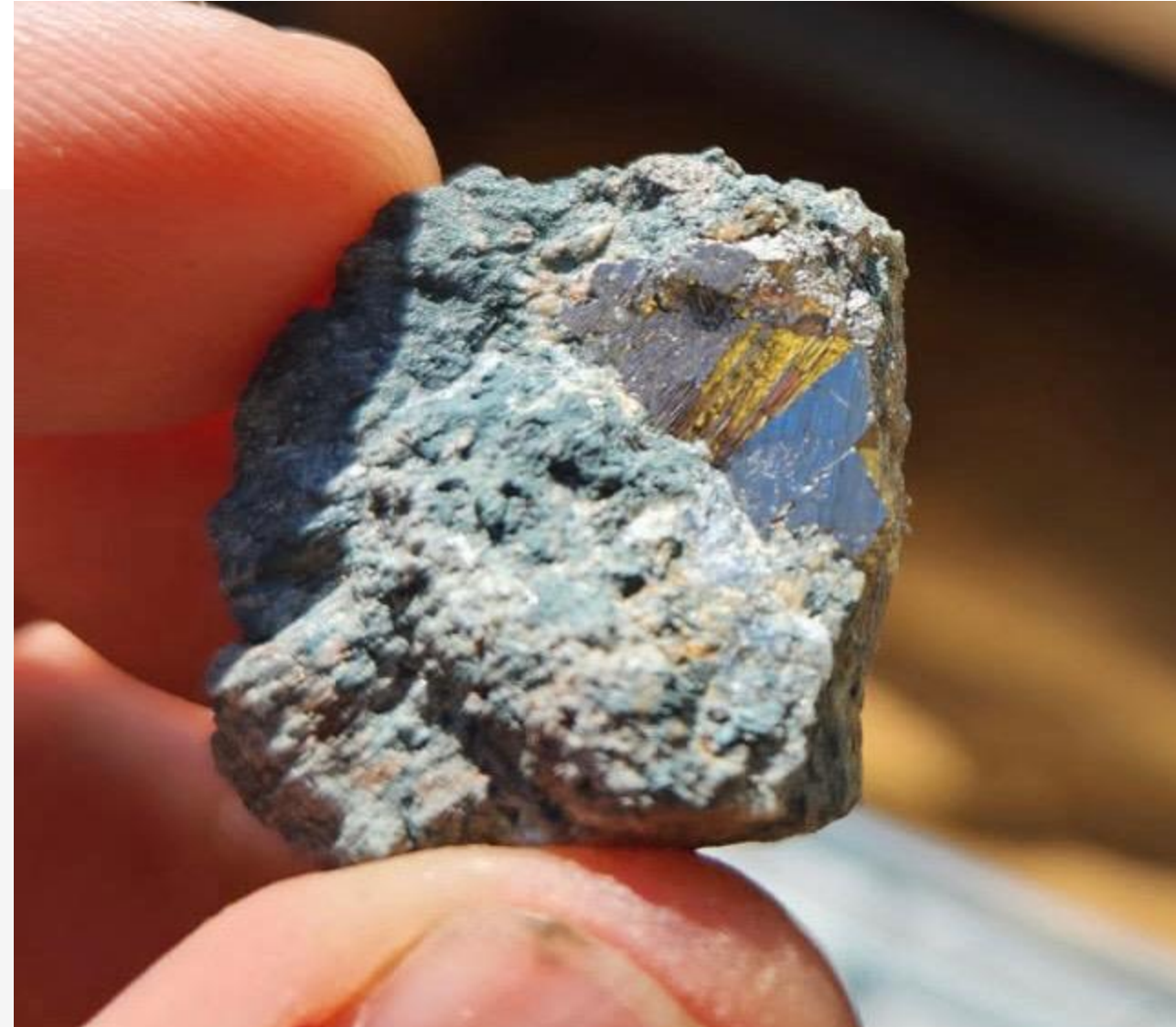
Rare arsenopyrite top right, encountered in first hole at approximately 330 m in depth
