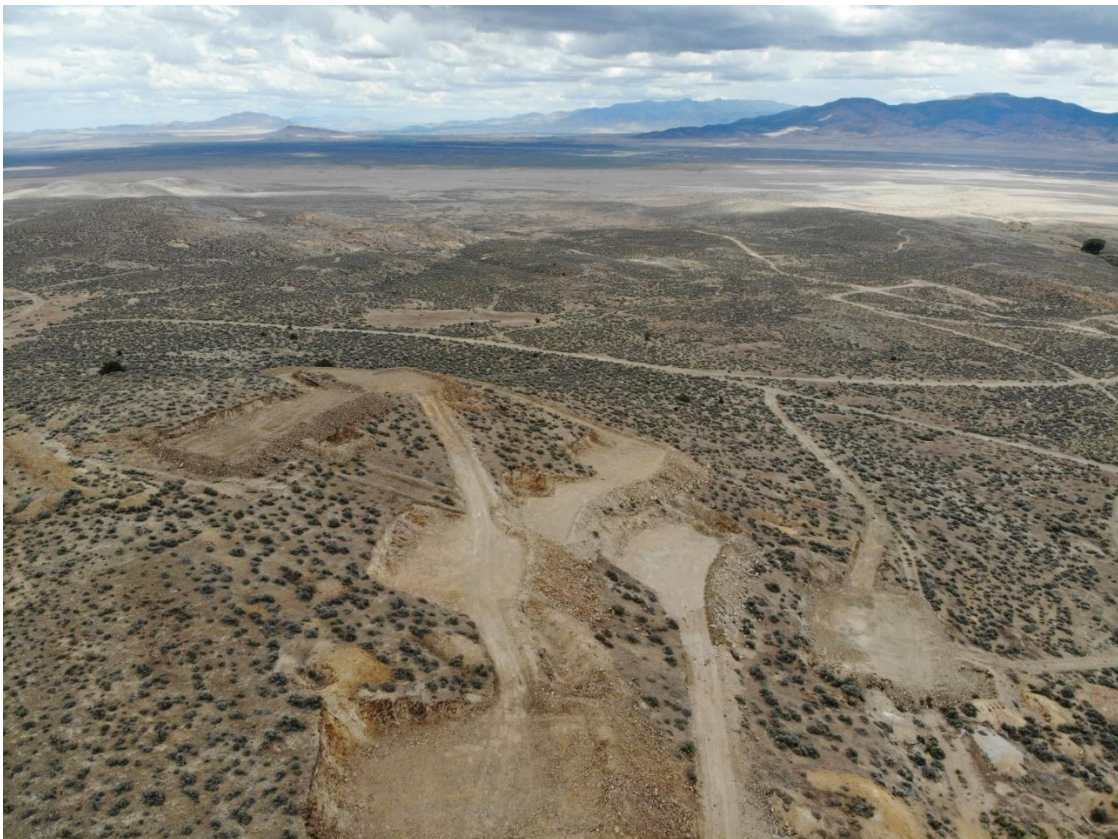
Figure 3: Aerial view of the Keystone Mine, with pads prepared for upcoming drilling campaign. Historic Keystone Mine workings can be seen in the lower left, along the north striking main Keystone Vein.
