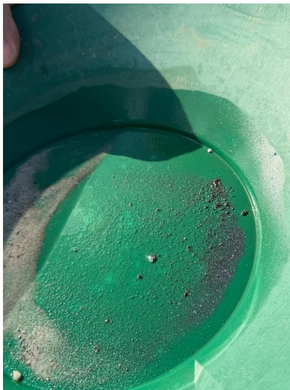
Figure 4: Panned sulphide tail including sphalerite, tetrahedrite and galena ( \pm native silver) from approximately 400 grams of dump sample material; Keystone Project.
