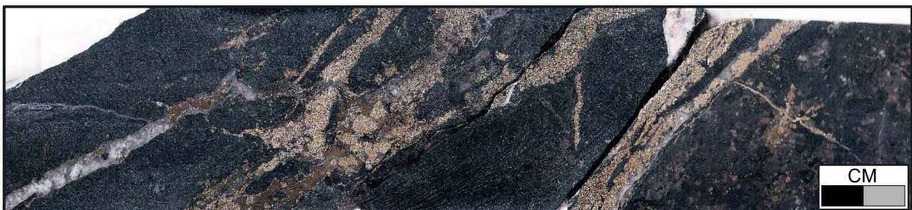
Figure 4: SPD038 97.2 m. - 13.5 g/t Au. Basalt with Quartz-pyrite, pyrite-chalcopyrite and quartz-pyrrhotite-pyrite veining
