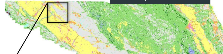
Mineral map from high resolution micro-XRF scan
