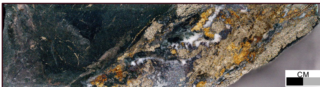
Figure 6: SPD045 - 137.2m, 12.43 g/t Au. Pyrite-chalcopryrite-galena-quartz vein in basalt
