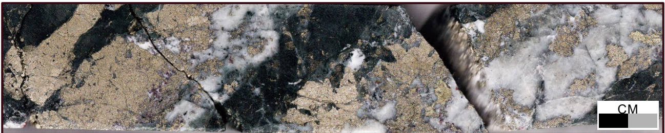
Figure 3: SPD031 - 739.3 m, 22.82 g/t Au . Pyrite-quartz-carbonate-chalcopyrite vein in basalt.
